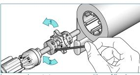
Loosen relevant stopper screws with an Allen key. Lengthen left back and right operated front roll shades by slightly turning and moving the inner stopper towards the clutch (1). Shorten the shade by turning and moving the inner stopper away from the clutch (2).
