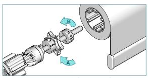
Lengthen right back and left operated front roll shades by slightly turning and moving the outer stopper away from the clutch (A). Shorten the shade by turning and moving the outer stopper towards the clutch (B).
