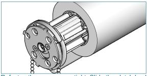
Refasten the screws very tight. Slide the clutch back into the tube.
