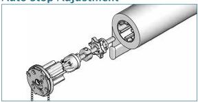
Remove the roller shade. Take out the clutch.
