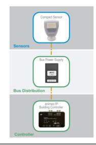
4. Powering devices during configuration: The Bus Power Supply can be used for temporary power while configuring SDN components such as Keypads and RTS Receivers. Simply connect a USB to RS485 adapter (#9015260) to the SDN data pass-through input and the device to be programmed to the SDN Power/Data output.
