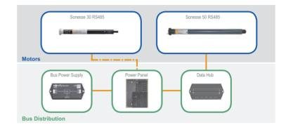
**3. Powering animeo IP<sup>®</sup> sensors:** The Bus Power Supply can be used to power the animeo IP Compact Sensor or Sensor Station. Connection is made from the Building Controller or Sub Controller sensor bus output to the Bus Power Supply's pass-through input. Then connect Compact Sensor or Sensor Station's outdoor sensor box to Bus Power Supply SDN Power /Data output
