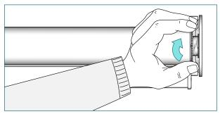
Secure the shade by turning the locking ring on the tube bearing plug furthest away from the bracket.
