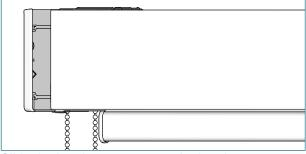
Slide the bracket covers onto the brackets.
