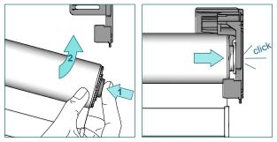
Press the tube bearing plug and lift the shade until it snaps into the bracket.
