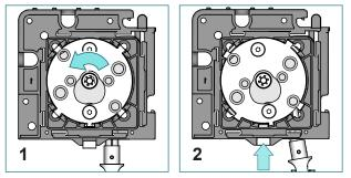
Insert the crank with the front plate into the bracket (1). Turn the crank in the rolling off direction and secure it with the locking clip (2).
