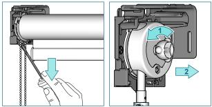
Place the screw driver into the slot of the locking clip. Press the locking clip down and turn the crank in the roll-up direction. Take the crank out of the bracket.
