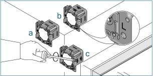
Install the brackets (L or R marked inside) with the screws provided. a) recess b) ceiling c) wall
