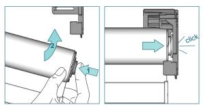
Press the tube bearing plug, lift the roller shade and snap it into the bracket.
