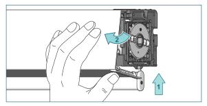
Press the bottom of the fascia upwards (1) and pull it outwards (2).
