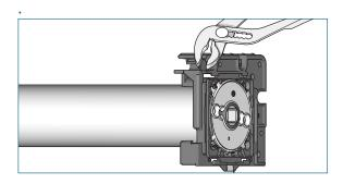
Use a pair of pliers to break off the stopper from the intermediate bracket.
