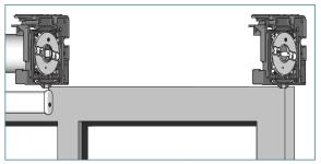
Install the outer bracket with the screws provided.
