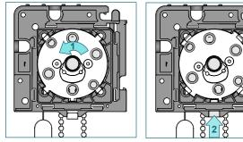
Turn the shade (10°) in the rolling off direction (1) and secure it with the locking clip (2).
