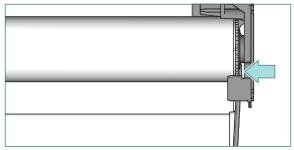
Unfasten the locking ring. Slide a screw driver between locking ring and bracket and push the tube bearing plug in the aligner/connector direction.
