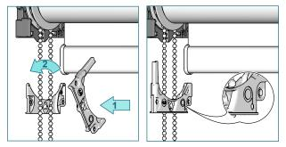
Put the chain between the chain outlet. Pay attention that stamping and roll-off direction of the shade are identical. Put the parts together (1) and turn left for closing (2).
