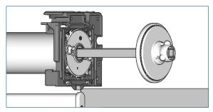
Slide the aligner or the connector set through the intermediate bracket into the tube bearing plug.
