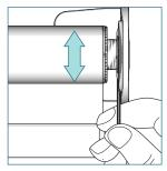
To adjust skewing, put the provided Allen key into the screw of the leveler and turn it left or right to move the shade up and down. Support lifting of large heavy roller shades with the palm of your hand.
