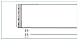
Slide the bracket covers onto the brackets.
