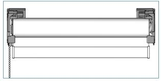
...line up teeth of the clutch with bracket & insert
