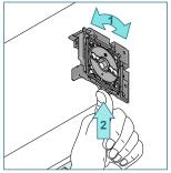
Insert the Plate L into the bracket on the idle end side. Turn the Plate L in the rolling off direction (1) and secure with the locking clip (2).
