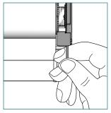
To adjust skewing, put the provided Allen key into the screw of the leveler and turn it left or right to move the shade up and down. Support lifting of large heavy shades with the palm of your hand.
