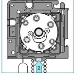
Turn the shade (10°) in the rolling off direction (1) and secure it with the locking clip (2).
