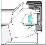
Slide the chain outlet up to the clutch and attach on the bracket with the 2 screws provided. Secure the shade by turning the locking ring away from bracket.
