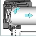
Open fastener on bracket adapter. Place the screwdriver into the slot of the bracket clip & slide the clip down and turn the shade in the roll-up direction.
