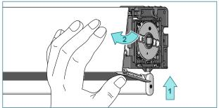
Press the bottom of the fascia upwards (1) and pull it outwards (2). Loosen both screws from the chain outlet and remove the outlet.
