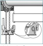
Put the chain between the chain outlet. Pay attention that stamping and roll-off direction of the shade are identical. Put the parts together (1) and turn left for closing (2).
