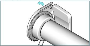
Lift the backside of the bracket cover ...
