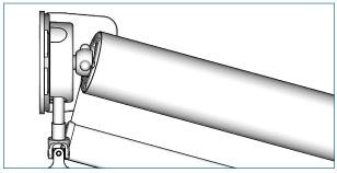
Place the tube adapter on the crank head.
