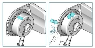
Slide the crank into the bracket adapter, turn it  $(10^{\circ})$  in the rolling off direction (1). Close fastener to secure the crank.(2)
