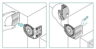
Slide the screw cover onto the bracket until it snaps. The fastener on the bracket adapter must be open.
