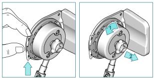
Open the fastener of the bracket adapter. Turn the crank in the roll up direction until the crank can be pulled out of the bracket adapter.
