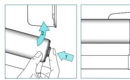
Press the tube bearing plug (1), lift the shade and snap into the bracket.
