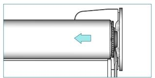
Unfasten the locking ring. Slide a screw driver between locking ring and bracket and push the tube bearing plug in the crank direction.
