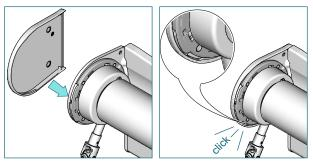
Slide the bracket covers onto the brackets. Make sure the bracket covers snap onto the brackets.
