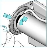
Line up teeth of motor Plate L with the bracket adapter (A). Turn the shade (10°) in the rolling off direction (1) close fastener on the bracket adapter (2). Make sure that limit switches are accessible on motors.
