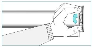
Secure the shade by turning the locking ring furthest away from the bracket.
