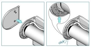
Slide the bracket covers onto the brackets. Make sure that the bracket covers snap onto the brackets.
