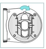
Make sure that the opening for the Allen key is pointing downwards before installing the brackets. Change the orientation by loosening the 4 screws and turning the leveler 90°. Reinstall the screws.
