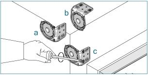
Install the brackets with the screws provided. a) recess b) ceiling c) wall
