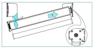
Place the shade with the tube bearing plug onto the bracket. (1) Push the shade against the idle end and lift the shade up (2).
