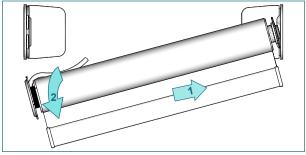
Push the shade against the tube bearing plug and slide it out of the bracket.
