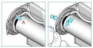
Line up teeth of motor Plate L with the bracket adapter (A).Turn the shade (10°) in the rolling off direction (1) close fastener on the bracket adapter (2). Make sure that limit switches are accessible on motors.
