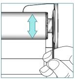
To adjust skewing, put the provided Allen key into the screw of the leveler and turn it left or right to move the shade up and down. Support lifting of large heavy shades with the palm of your hand.
