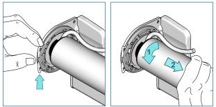
Open fastener on the bracket adapter. Turn the shade in the roll up direction (1) and then pull Plate L out of the bracket adapter.(2)
