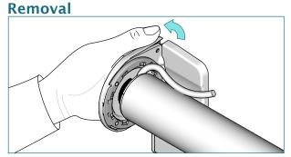
Disconnect power to the motor. Lift the backside of the bracket cover...
