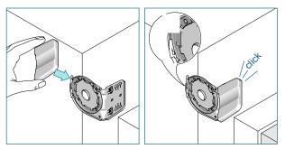
Slide the bracket cover onto the bracket until it snaps. The fastener of the bracket adapter must be open.
