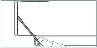
Disconnect power to the motor. Place the screw driver under the bracket cover, turn the screw driver and slide the bracket cover from the bracket.
