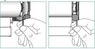
To adjust skewing, put the provided Allen key into the screw of the leveler and turn it left or right to move the shade up and down. Support lifting of large heavy shades with the palm of your hand.
