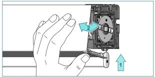
Press the bottom of the fascia upwards (1) and pull it outwards (2).
