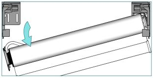
Push the shade against the tube bearing plug and slide it out of the bracket.
