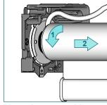
Unfasten the locking ring. Place the screw driver into the slot of the locking clip. Press the locking clip down and turn the shade in the roll-up direction.
