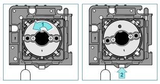
Turn the shade (10°) in the rolling off direction (1) and secure it with the locking clip (2).
