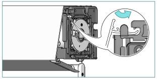
Place the fascia in the bracket. Make sure that the fascia slides under the nose of the bracket.
