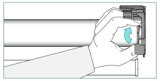
Secure the shade by turning the locking ring on the tube bearing plug furthest away from the bracket.
