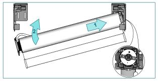
Place the shade with the tube bearing plug onto the bracket. Push the shade against plug and lift up...
