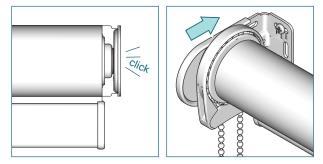
Snap it to the bracket. Slide the bracket covers on to the brackets.
