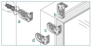
Install the brackets with the screws provided.
