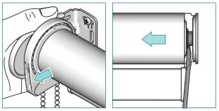
Slide a screw driver between tube bearing plug and bracket and push the bearing in the clutch direction. Slide the bracket cover towards you.
