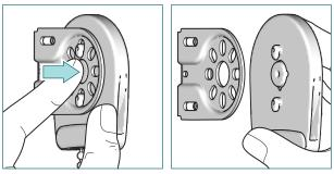
Push the pin of the clutch and take the clutch out of the bracket.
