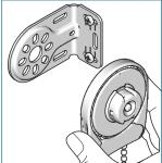
Place a screw driver under the pin of the clutch and pull it outwards. Take the clutch out of the bracket.
