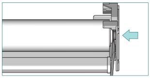
Slide a screw driver between the tube bearing plug and bracket and push the plug in the clutch direction.
