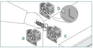
Install the brackets (L or R marked inside) with the screws provided.
