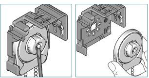
Place a screw driver under the pin of the clutch and pull it outwards. Take the clutch out of the bracket.
