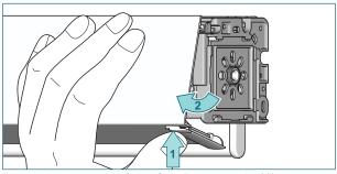
Press the bottom of the fascia upwards (1) and then pull it outwards (2).
