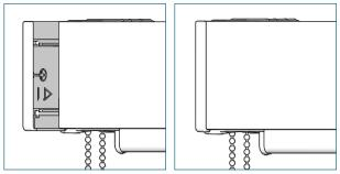
Slide the bracket covers onto the brackets.
