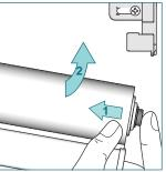
Place the tube on to the clutch head. Press the tube bearing plug (1), lift the shade & snap into bracket (2).
