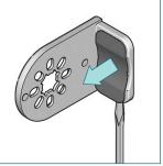
Press the bracket cover out of the decorator bracket. Use a screw driver to remove the screw cover cap from the decorator bracket.
