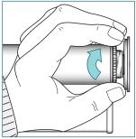
Snap it to the bracket. Secure the shade by turning the locking ring furthest away from the bracket.
