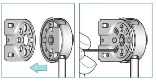
Place the crank in the bracket and attach both screws.
