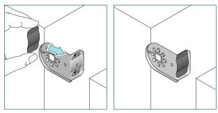
When using decorator brackets, slide the screw cover cap onto the bracket until it snaps.
