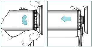
Unfasten the locking ring. Slide a screw driver between locking ring and bracket and push the tube bearing plug in the crank direction.
