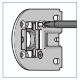
Make sure that the opening for the Allen key is pointing downwards before installing the brackets. Change the orientation by loosening the 2 screws and turning the leveler 90°. Reinstall the screws.
