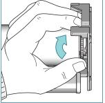
... until it snaps into the bracket. Secure shade by turning the locking ring furthest away from the bracket.
