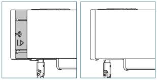
Slide the bracket covers onto the brackets.
