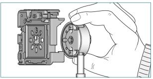
Loosen both screws and take the crank out of the bracket.
