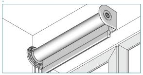
Make sure the bracket cover is on the intermediate plug bracket.
