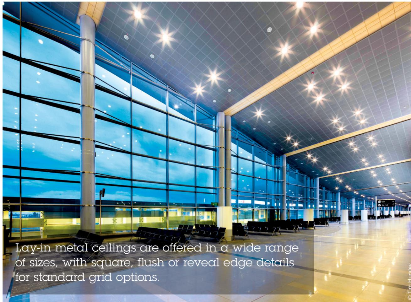
Lay-in metal ceilings are offered in a wide range of sizes, with square, flush or reveal edge details for standard grid options.
