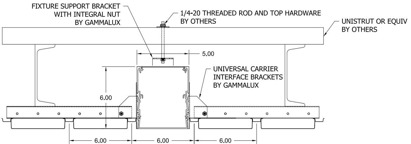
**Mounting bracket is field adjustable to accommodate Box 6 or Deep Box 6 conditions.**
