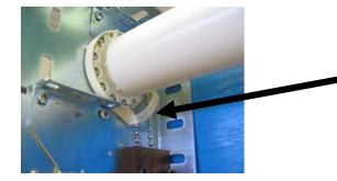
**Note-** Make sure the clutch is rotated 45° to ensure smooth functionality of the chain while being rotated through the guide.
