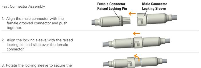
3. Rotate the locking sleeve to secure the connectors together.
