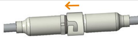
3. Rotate the locking sleeve to secure the connectors together.
