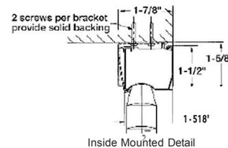
Note: Headrail and brackets are the same for both Mark I 1-3/8" and Mark I 1" products.
