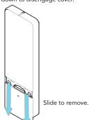
Install battery with positive (+) side facing up.
