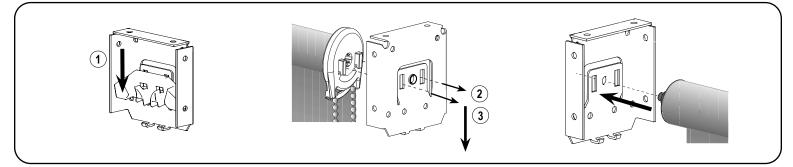
First, attach chain diverter into the clutch bracket by gently pulling down. Insert the hooks on the clutch straight into the two slots in the bracket. Once the two hooks are through the slots, gently pull down on the clutch until the hooks have locked securely to the bracket. Then, place the spring loaded pin end into the round hole of the bracket.
