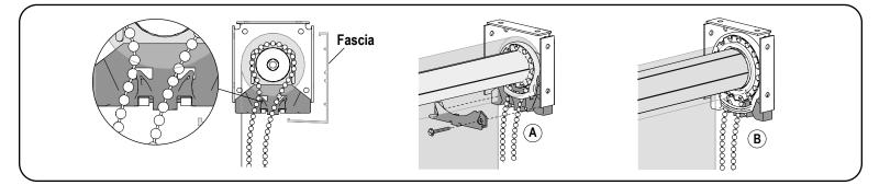
Once the roll has been installed, align the chain in the diverter as shown. This allows room for fascia attachment. For SL10 & SL15 (A), attach the chain diverter cover. If needed, secure the cover with screws. The Clutch SL20 (B) does not require a cover.
