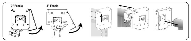
First, rotate upward to disengage the fascia. Then, gently pull up the control unit (Clutch, Motor or Spring) until the hooks touch the top part of the bracket slot. Pull the shade towards the spring loaded pin end until the hooks are complete out of the bracket slots. Finally, remove the spring loaded pin end from the idler bracket.
