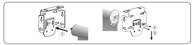
First, place the spring loaded pin end into the round hole of the bracket. Then, keeping the pin end secure in its bracket, insert the hooks on the clutch straight into the two slots in the bracket. Once the two hooks are through the slots, gently pull down on the clutch until the hooks have locked securely to the bracket. The bottom of the clutch should point straight down.
