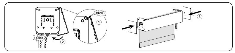
First, position the fascia top ridge into the front top channel of all brackets. Then, rotate the bottom front of the fascia downwards until the bottom rear of the fascia snap into the bracket. Finally, attach the bracket covers.
