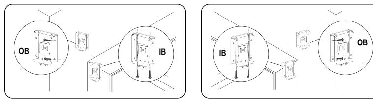
**Inside Mount (IB)**, Install each bracket with two screws either through the side or up through the top. Make sure all brackets are leveled and aligned. **Outside Mount (OB)**, Secure each bracket with two screws. Make sure all brackets are level. Minimum 1 1/4" mounting surface height requirement.
