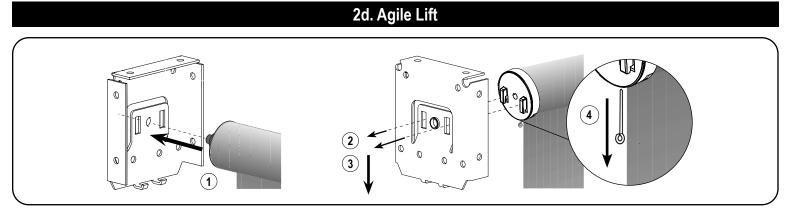
Important: Do not to pull the lock pin until shade is securely assembled onto the brackets.
