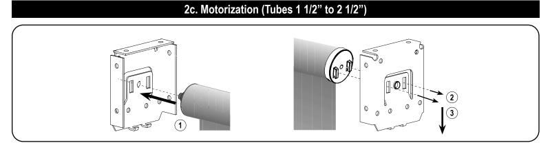
First, place the spring loaded pin end into the round hole of the bracket. Then, keeping the pin end secure in its bracket, insert the hooks on the motor head straight into the two slots in the bracket. Once the two hooks are through the slots, gently pull down on the motor until the hooks have locked securely to the bracket. The bottom of the motor head should point straight down.
