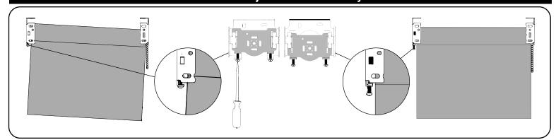
Note: In some installations, due to leveling issues, the shade may "telescope". This is not considered a defect.
