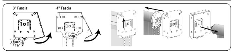
First, rotate upward to disengage the fascia. Then, gently pull up the control unit (Clutch, Motor or Spring) until the hooks touch the top part of the bracket slot. Pull the shade towards the spring loaded pin end until the hooks are complete out of the bracket slots. Finally, remove the spring loaded pin end from the idler bracket.
