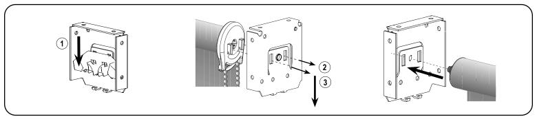
First, attach chain diverter into the clutch bracket by gently pulling down. Insert the hooks on the clutch straight into the two slots in the bracket. Once the two hooks are through the slots, gently pull down on the clutch until the hooks have locked securely to the bracket. Then, place the spring loaded pin end into the round hole of the bracket.
