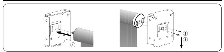
First, place the spring loaded pin end into the round hole of the bracket. Then, keeping the pin end secure in its bracket, insert the hooks on the motor head straight into the two slots in the bracket. Once the two hooks are through the slots, gently pull down on the motor until the hooks have locked securely to the bracket. The bottom of the motor head should point straight down.
