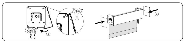
First, position the fascia top ridge into the front top channel of all brackets. Then, rotate the bottom front of the fascia downwards until the bottom rear of the fascia snap into the bracket. Finally, attach the bracket covers.
