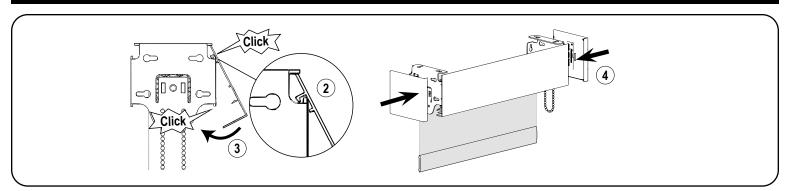
First, position the fascia top ridge into the front top channel of all brackets. Then, rotate the bottom front of the fascia downwards until the bottom rear of the fascia snap into the bracket. Finally, attach the bracket covers.
