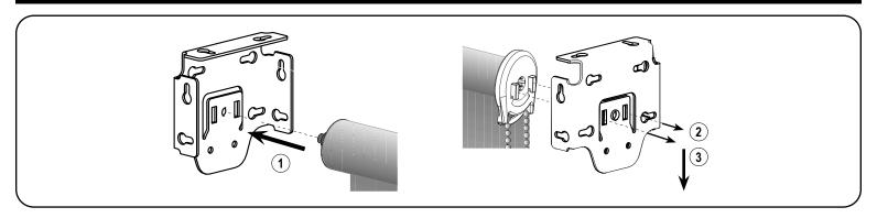
First, place the spring loaded pin end into the round hole of the bracket. Then, keeping the pin end secure in its bracket, insert the hooks on the clutch straight into the two slots in the bracket. Once the two hooks are through the slots, gently pull down on the clutch until the hooks have locked securely to the bracket. The bottom of the clutch should point straight down.
