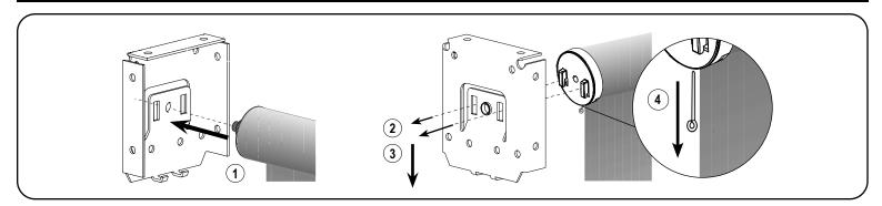
**Important:** Do not to pull the lock pin until shade is securely assembled onto the brackets.
