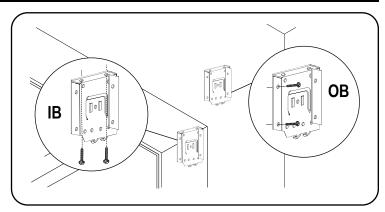
Inside Mount (IB), Install each bracket with two screws either through the side or up through the top. Make sure all brackets are leveled and aligned.
