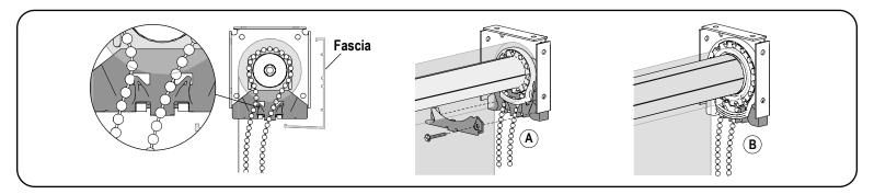
Once the roll has been installed, align the chain in the diverter as shown. This allows room for fascia attachment. For SL10 & SL15 (A), attach the chain diverter cover. If needed, secure the cover with screws. The Clutch SL20 (B) does not require a cover.
