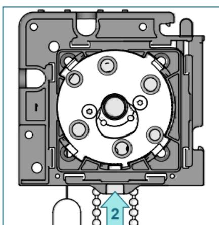
Turn the shade (10°) in the rolling off direction (1) and secure it with the locking clip (2).
