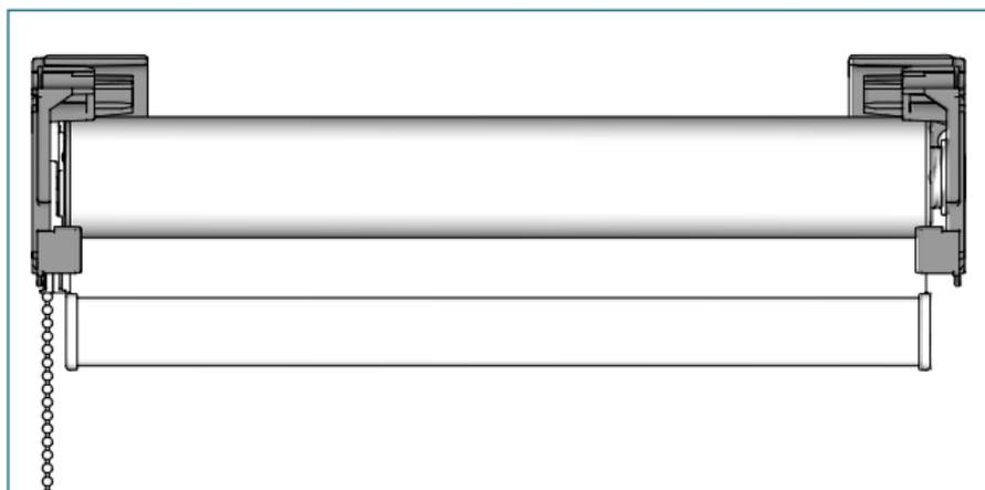
...line up teeth of the clutch with bracket and insert.
