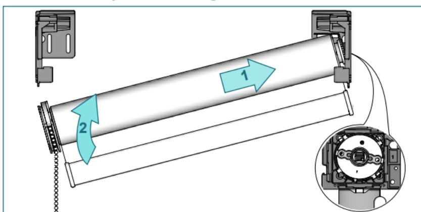
Place the shade with the idle end onto the bracket. Push the shade against tube bearing plug and lift it up ...
