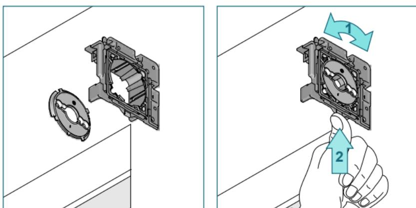
Insert the Plate L into the intermediate bracket. Turn the Plate L in the rolling off direction (1) and secure with the locking clip (2).
