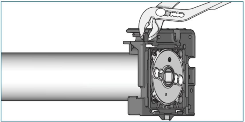
Use a pair of pliers to break off the stopper from the intermediate bracket.
