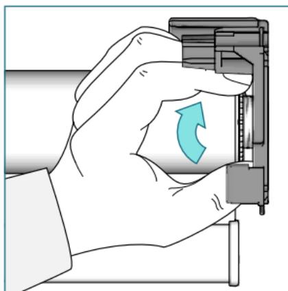
Slide the chain outlet up to the clutch and attach on the bracket with the 2 screws provided. Secure the shade by turning the locking ring away from the bracket.
