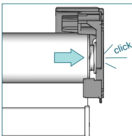
Press the tube bearing plug, lift the roller shade and snap it into the bracket.
