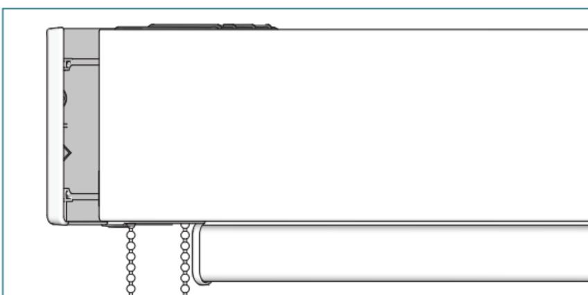
Slide the bracket covers onto the brackets.
