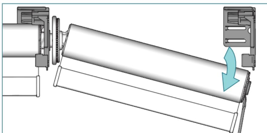
Move the roller shade downwards out of the bracket. Pull the aligner or connector out of the idle end.
