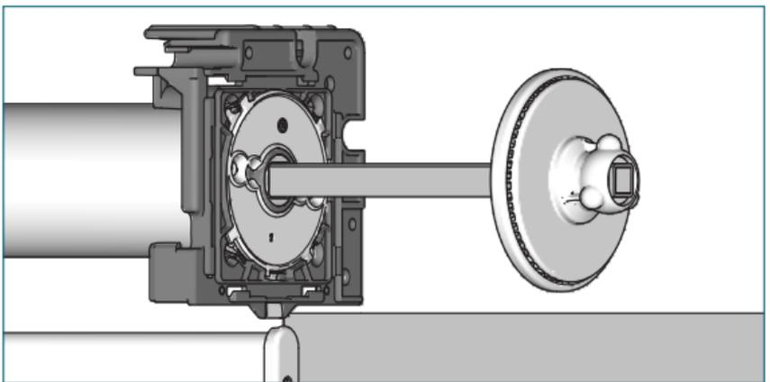
Slide the aligner or the connector set through the intermediate bracket into the tube bearing plug.
