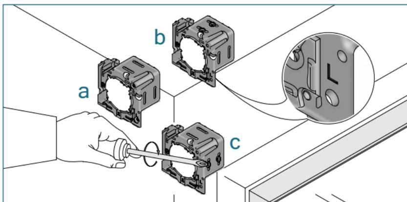
Install the clutch bracket and intermediate bracket first.
