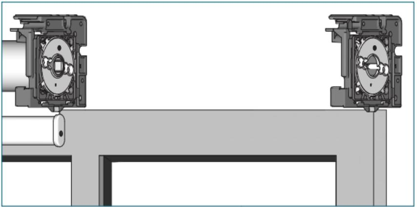
Install the outer bracket with the screws provided.
