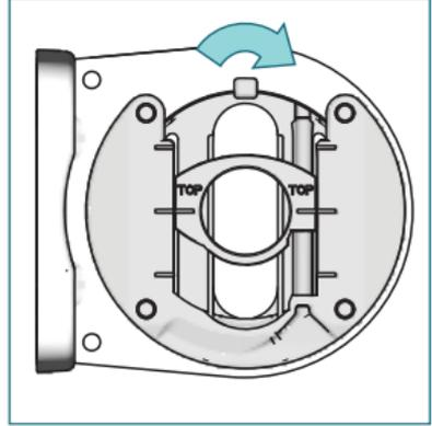
Make sure that the opening for the Allen key is pointing downwards before installing the brackets. Change the orientation by loosening the 4 screws and turning the leveler 90°. Reinstall the screws.
