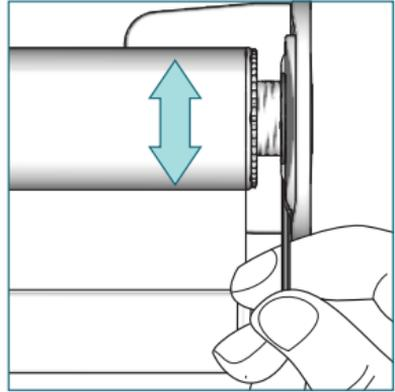
To adjust skewing, put the provided Allen key into the screw of the leveler and turn it left or right to move the shade up and down. Support lifting of large heavy roller shades with the palm of your hand.
