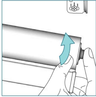
Insert the tube on to the clutch head. Press the tube bearing plug and lift the shade.
