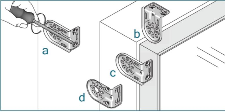
Install the brackets with the screws provided.
