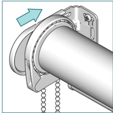
Snap it to the bracket. Slide the bracket covers on to the brackets.
