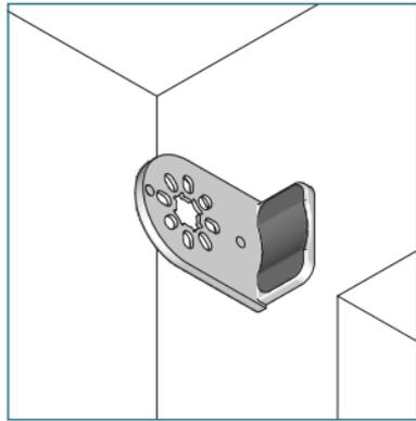
When using decorator brackets, slide the screw cover cap onto the bracket until it snaps.
