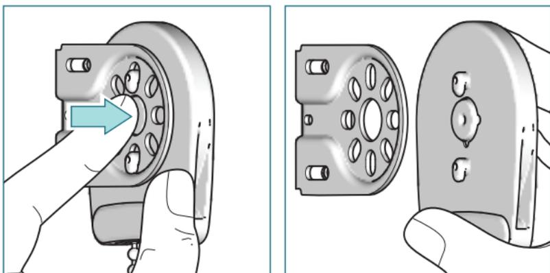
Push the pin of the clutch and take the clutch out of the bracket.
