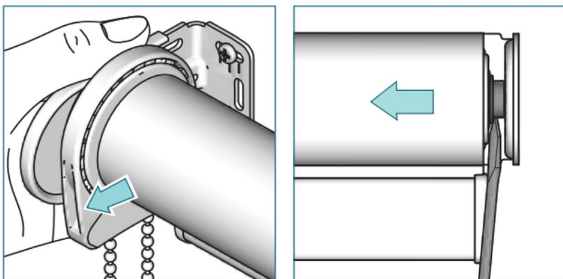
Slide a screw driver between tube bearing plug and bracket and push the bearing in the clutch direction. Slide the bracket cover towards you.
