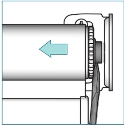
Unfasten the locking ring. Slide a screw driver between locking ring and bracket and push the tube bearing plug in the crank direction.
