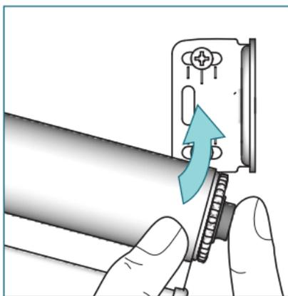
Place the tube on to the crank head. Press the tube bearing plug and lift the shade.
