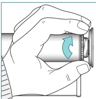
Snap it to the bracket. Secure the shade by turning the locking ring furthest away from the bracket.
