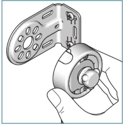
Loosen both screws and take the crank out of the bracket.
