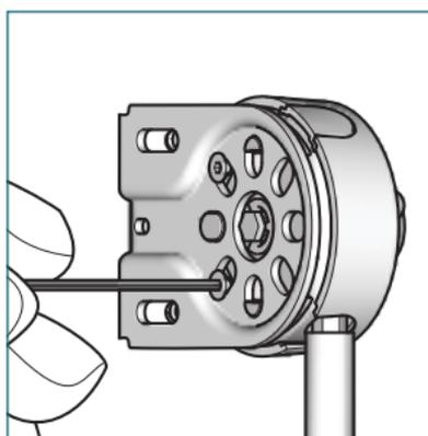
Place the crank in the bracket and attach both screws.
