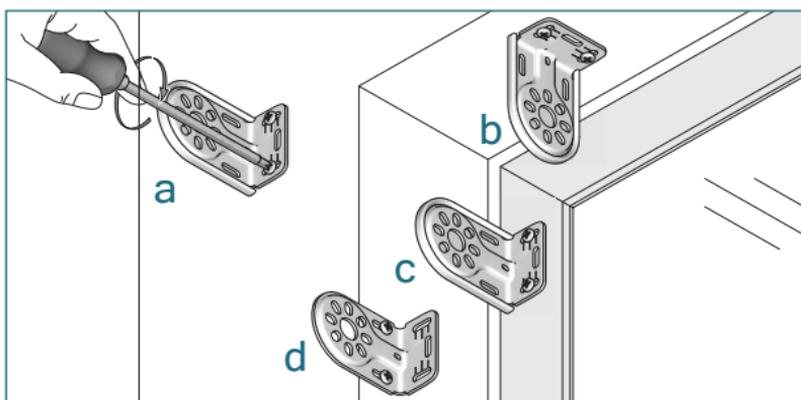
Install the brackets with the screws provided.
