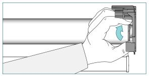
Secure shade band by turning the locking ring on tube bearing plug furthest away from the bracket.
