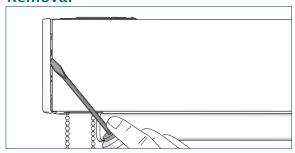
Place the screw driver under the bracket cover, turn the screw driver and slide the bracket cover from the bracket.
