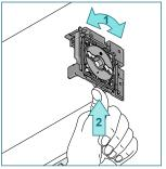
Insert the Plate L into the intermediate bracket. Turn the Plate L in the rolling off direction(1) and secure with the locking clip (2).
