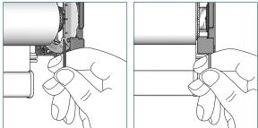
To adjust skewing, put the provided Allen key into the screw of the leveler and turn it left or right to move the shade up and down. Support lifting of large heavy roller shades with the palm of your hand.
