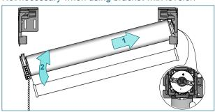
Place the shade with the idle end onto the bracket. Push the shade against tube bearing plug and lift it up ...
