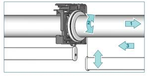
To align the bottom hembars, pull the shade away from aligner set (1), turn shade to line up bottom hembars together (2). Release shade to secure position (3). Not possible when using connector set.
