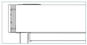
Slide the bracket covers onto the brackets.
