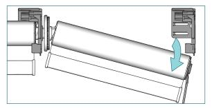
Move the roller shade downwards out of the bracket. Pull the aligner or connector out of the idle end.
