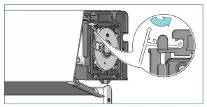
Place the fascia in the bracket. Make sure that the fascia slides under the nose of the bracket.
