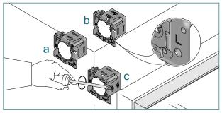
Install the clutch bracket and intermediate bracket first.
