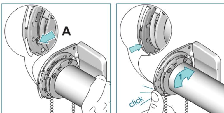
Line up teeth of the clutch with bracket adapter (A). Insert clutch, turn shade (10°) in the rolling off direction (1), and close fastener on the bracket adapter.
