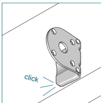
Slide the screw cover onto the bracket until it snaps.
