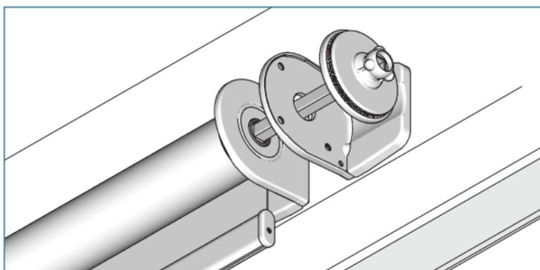
Shades with custom width gaps or Joint 45° will require 2 intermediate brackets. Slide the aligner or connector set through the intermediate bracket into the tube bearing plug.
