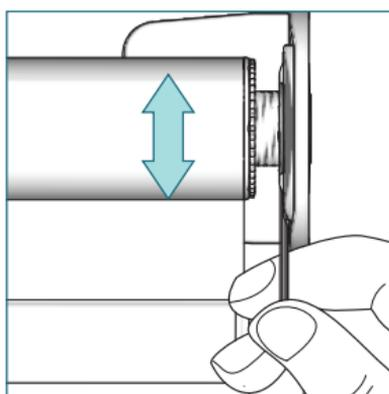
To adjust skewing, put the provided Allen key into the screw of the leveler and turn it left or right to move the roller shade up and down. Support lifting of large heavy roller shades with the palm of your hand.
