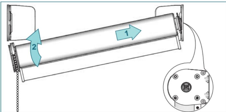
Place the roller shade with the idle end onto the intermediate bracket. Push the shade against the tube bearing plug and lift the shade into the clutch bracket.
