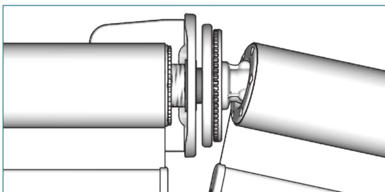
Place the tube with plug connector on the aligner or connector set head.
