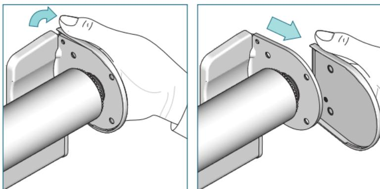
Lift the backside of the bracket cover and slide it towards you.
