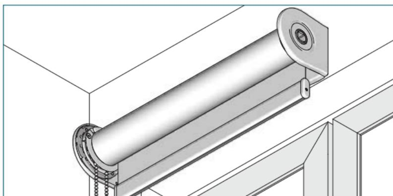
Make sure the bracket cover is on the intermediate plug bracket.
