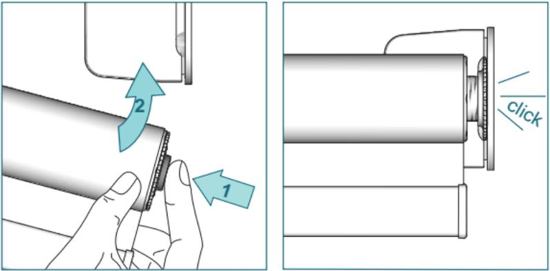
Press the tube bearing plug, lift the roller shade and snap it to the bracket.
