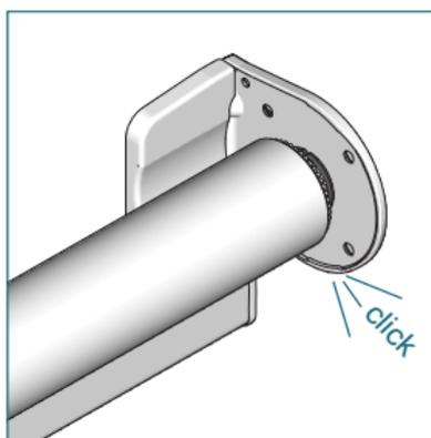
Slide the bracket cover onto the bracket. Make sure that the bracket cover snaps onto the bracket.
