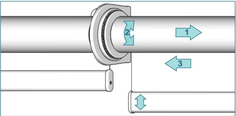
To align the bottom hembar, pull the shade away from aligner set (1), turn shade to line up bottom hembar together (2). Release shade to secure position (3). Not possible when using connector set.
