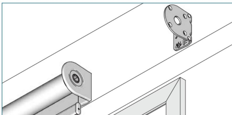
Install the end plug bracket with screws provided.
