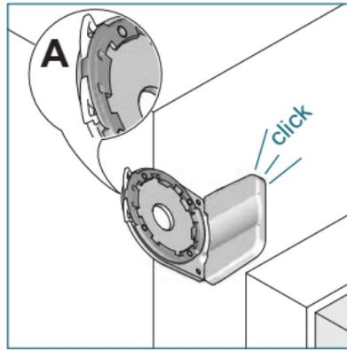
Slide the screw cover onto the bracket until it snaps. Open the fastener on the clutch bracket adapter (A).
