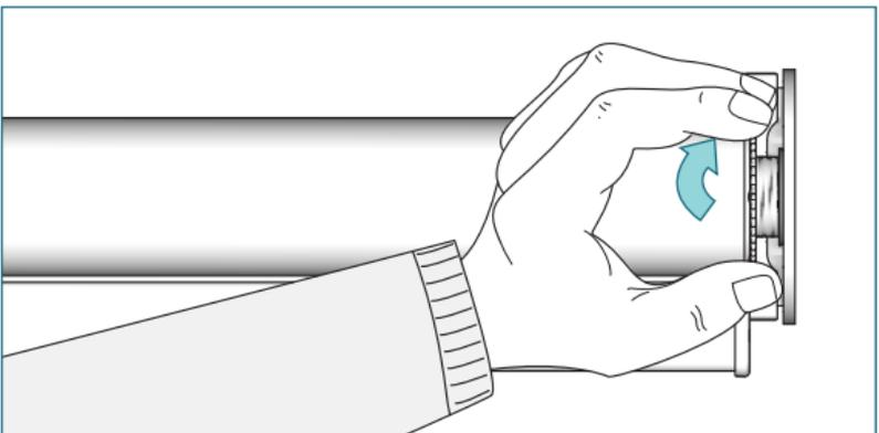
Secure shade band by turning the locking ring on tube bearing plug furthest away from the bracket.
