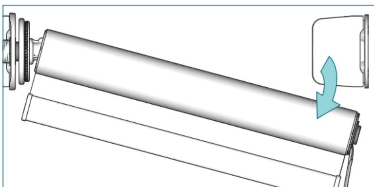
Move the roller shade downwards out of the bracket. Pull the aligner or connector out of the tube bearing plug.
