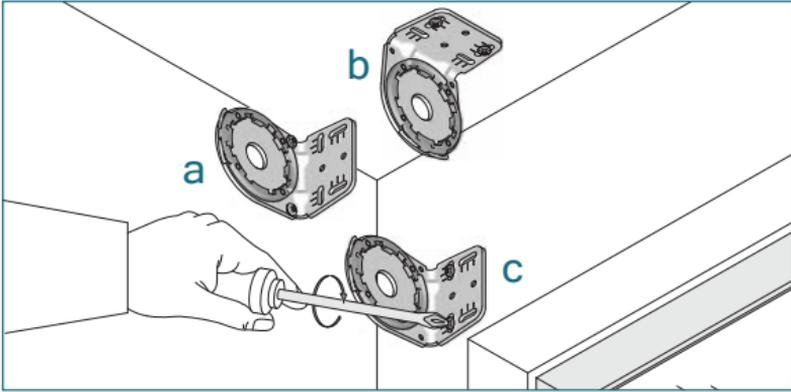
Install the clutch bracket & intermediate plug bracket first. a) recess b) ceiling c) wall
