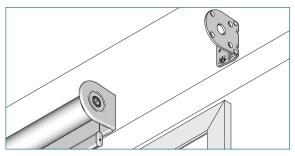
Install the end plug bracket with screws provided.
