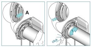
Line up teeth of the clutch with bracket adapter (A). Insert clutch, turn shade  $(10^{\circ})$  in the rolling off direction (1), and close fastener on the bracket adapter.
