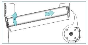
Place the roller shade with the idle end onto the intermediate bracket. Push the shade against the tube bearing plug and lift the shade into the clutch bracket.
