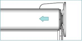
Unfasten the locking ring. Slide a screw driver between locking ring and bracket and push the tube bearing plug in the aligner/connector direction.
