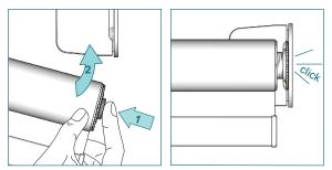
Press the tube bearing plug, lift the roller shade and snap it to the bracket.
