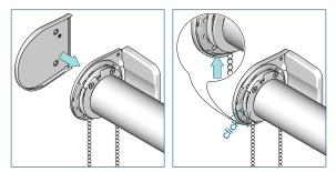
Attach the bracket covers onto the brackets. Make sure the bracket covers snap onto the brackets.
