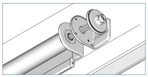
Shades with custom width gaps or Joint 45° will require 2 intermediate brackets. Slide the aligner or connector set through the intermediate bracket into the tube bearing plug.
