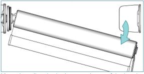
Move the roller shade downwards out of the bracket. Pull the aligner or connector out of the tube bearing plug.
