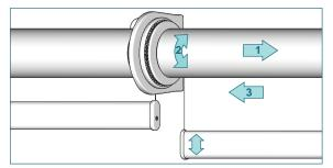
To align the bottom hembars, pull the shade away from aligner set (1), turn shade to line up bottom hembars together (2). Release shade to secure position (3). Not possible when using connector set.
