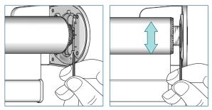
To adjust skewing, put the provided Allen key into the screw of the leveler and turn it left or right to move the roller shade up and down. Support lifting of large heavy roller shades with the palm of your hand.
