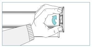
Secure the shade by turning the locking ring furthest away from the bracket.
