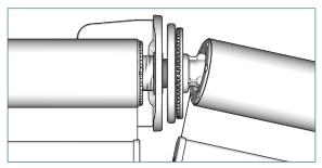
Place the tube with plug connector on the aligner or connector set head.
