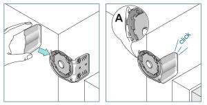
Slide the screw cover onto the bracket until it snaps. Open the fastener on the clutch bracket adapter (A).
