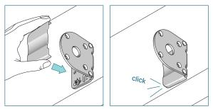
Slide the screw cover onto the bracket until it snaps.
