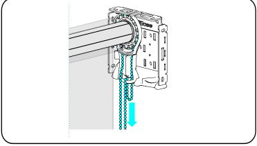
Pull Chain Through Diverter, Drop a loop of chain through the diverter and pull all of the chain through.
