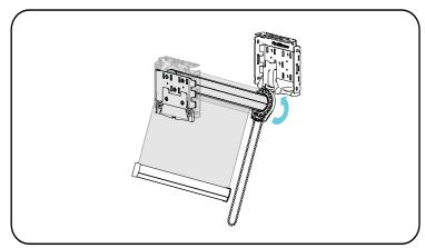
Attach Top Roller Assembly Pin First, Place the spring loaded pin end into the round hole of the bracket. Once the 2 hooks are through the slots, gently pull down on the clutch until the hooks have locked securely to the bracket. The bottom of the clutch should point straight down.
