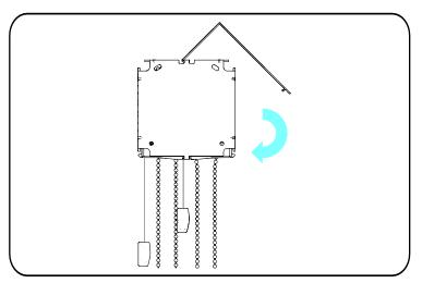
Attach the Fascia Panels, Flip the fascia so that the short side will mount to the top of the bracket. Align the hook to the bracket and rotate down over the face of the bracket system. Snap into locking position.
