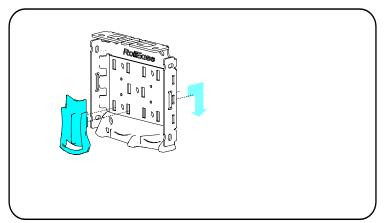
Attach Chain Diverter, Push hooks through the bracket and pull down.
