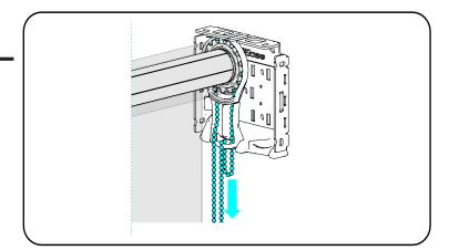
**Pull Chain Through Diverter**, Drop a loop of chain through the diverter and pull all of the chain through.
