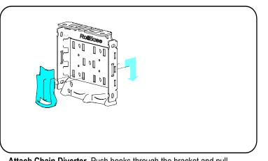
Attach Chain Diverter, Push hooks through the bracket and pull down.
