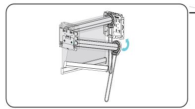
Attach Bottom Roller Assembly Pin First, Place the spring loaded pin end into the round hole of the bracket. Once the 2 hooks are through the slots, gently pull down on the clutch until the hooks have locked securely to the bracket. The bottom of the clutch should point straight down.
