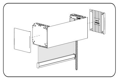
Attach Bracket Covers, Snap the bracket covers into the fascia
