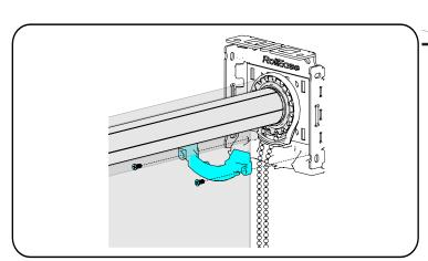
Attach the Chain Cover (Not required for SL30), Snap and screw the chain cover into place onto the chain diverter.
