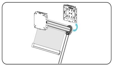
**Attach Top Roller Assembly Pin First,** Place the spring loaded pin end into the round hole of the bracket.
