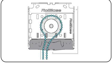
**Align Chain Through Diverter**, Move the chain toward the back through the diverter to allow fascia to attach.
