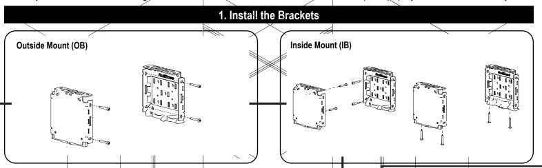
Inside Mount (IB). Install each bracket with two screws either through the side or up through the top. Make sure all brackets are leveled and aligned.
