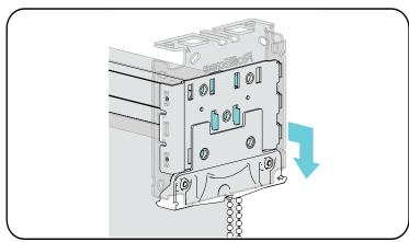
**Attach Clutch to Insert Plate,** Once the 2 hooks are through the slots, gently pull down on the clutch until the hooks have locked securely to the bracket. The bottom of the clutch should point straight down.
