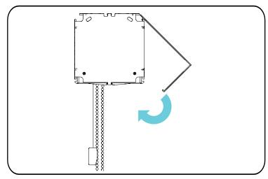
**Attach the Fascia Panels,** First, position the fascia top ridge into the front top channel of the bracket. Rotate the bottom front of the fascia downwards until the bottom rear of the fascia snaps in the bracket.
