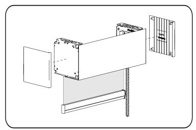
Attach Bracket Covers, Snap the bracket covers into the fascia bracket
