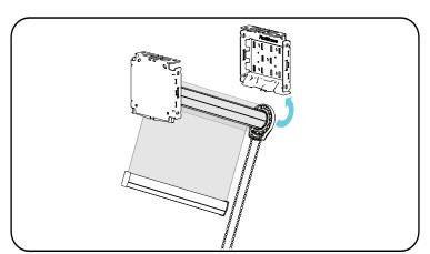
Attach Top Roller Assembly Pin First, Place the spring loaded pin end into the round hole of the bracket.
