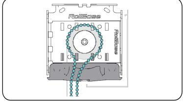
**Align Chain Through Diverter**, Move the chain toward the back through the diverter to allow fascia to attach.
