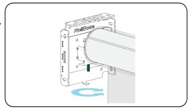
**Turn Screw to Adjust Shade Level**, Raise or lower the idle end of the shade to adjust the shade level by turning the adjustment screw clockwise or counterclockwise.
