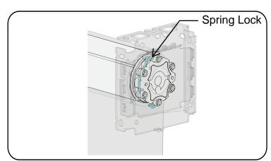
**Attach Motor to Insert Plate**, Keep the spring lock on the motor, align and press the motor into the motor plate on the bracket until the spring lock snaps into place.
