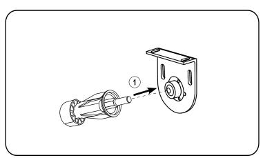
Attach the Pin End First, Place the spring loaded pin end into the round hole of the bracket.
