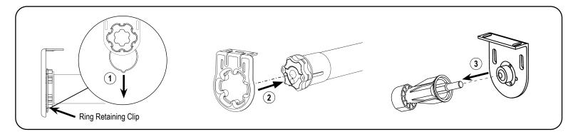
First, raise the shade. Remove the ring retaining clip in place from the motor. Then, slide the roll towards the spring loaded pin end until the motor head is completely out of the motor head slots. Lastly, remove the spring loaded pin end from the Idler bracket.
