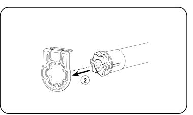
Attach Motor to Bracket, Align and press the motor into the motor plate on the bracket until the spring lock snaps into place.
