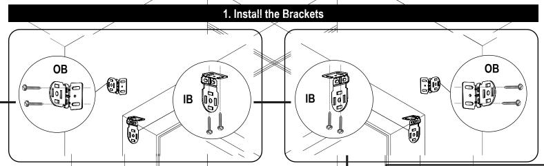
**Inside Mount (IB)** Install each bracket with two screws either through the side or up through the top. Make sure all brackets are leveled and aligned. **Outside Mount (OB)**, Secure each bracket with two screws. Make sure all brackets are level. Minimum 1 1/4" mounting surface height requirement.
