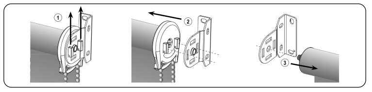
First, raise the shade. Gently lift up the control unit (hooks end) to disengage, until the hooks touch the top part of the bracket slot. Then, slide the roll towards the spring loaded pin end until the hooks are completely out of the bracket slots. Lastly, remove the spring loaded pin end from the Idler bracket.
