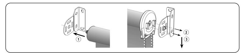
First, place the spring loaded pin end into the round hole of the bracket. Then, keeping the pin end secure in its bracket, insert the hooks on the clutch straight into the two slots in the bracket. Once the two hooks are through the slots, gently pull downward on the side with hooks until the hooks have locked securely to the bracket. The bottom of the clutch should point straight down.
