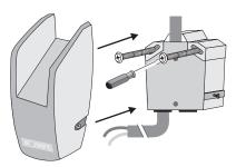
Attach the sensor to the wall.Replace front cover and secure with screws provided
