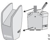
Loosen the strain relief plate and guide the power supply wires through the black grommet into terminal block.
