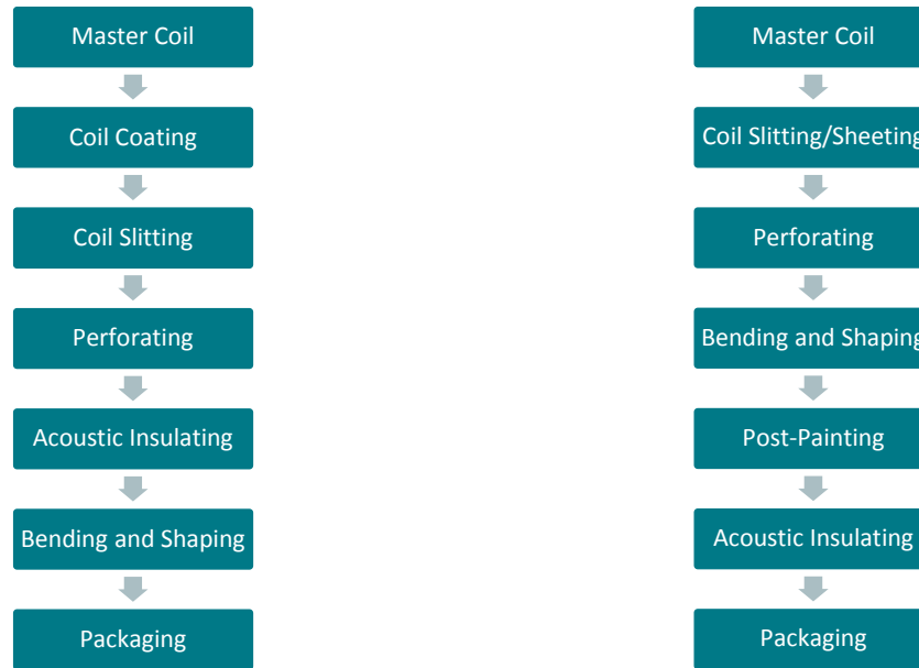
Figure 1: Typical aluminum specialty product manufacturing process, coil-coating (left) & post-paint (right)
